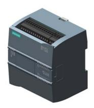
SIMATIC S7-1200, CPU 1212C, compact CPU, DC/DC/DC, onboard I/O: 8 DI 24 V DC; 6 DO 24 V DC; 2 AI 0-10 V DC, Power supply: DC 20.4-28.8V DC, Program/data memory 50 KB
